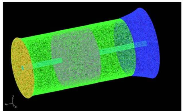
**Figure 2.3** Mesh of the Outer Volume
