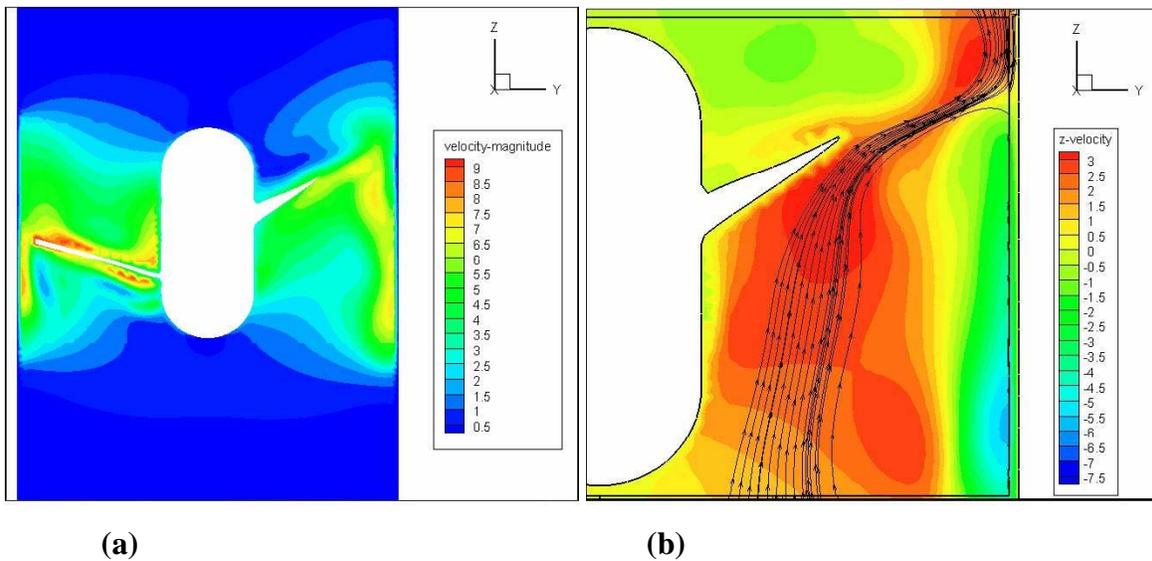
**Figure 4.3** Velocity contours on x-plane
